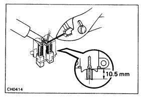
(c) Solder the brush wire to the brush holder at the exposed length.
