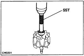
(b) Using SST and a press, press in a new bearing and the bearing cover.
