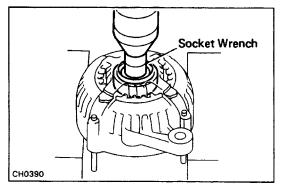
(b) Using a press and socket wrench, press out the front bearing.
