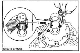
(c) Tighten the five screws until there is a clearance of at least 1 mm (0.04 in.) between the brush holder cover and connector.
